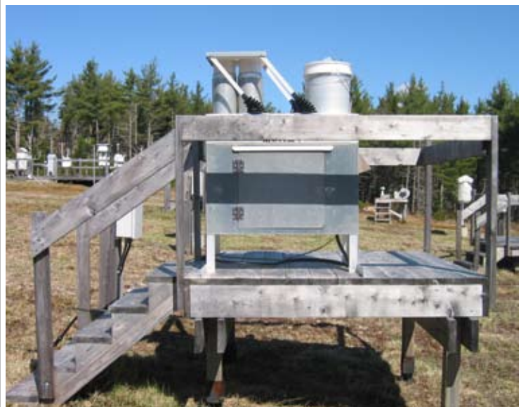
Mercury in precipitation collector (Photo by Environment Canada)
