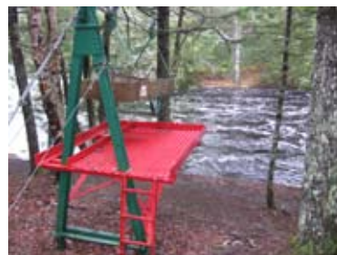
Stream flow sampling cables (Photo by D. Ure, Parks Canada)
