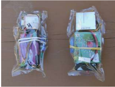
GPS logger units, with radio transmitter, packaged in 12 gauge vinyl.
