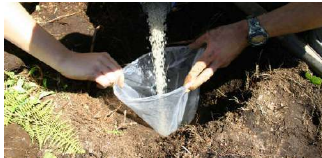
Measuring the volume of a soil sample
