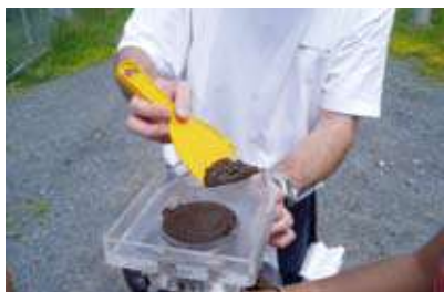
Sectioning a sediment core into 0.25 cm intervals on shore
