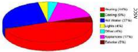
Breakdown of MTRI field station's energy consumption by type of use in 2009 shows that heating, hot water, and appliances consume 88% of the total energy budget
