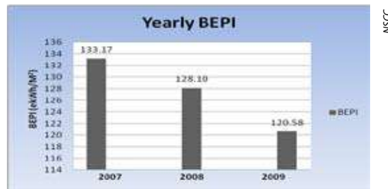
MTRI field station annual BEPI (building energy performance index) adjusts for the total square meters of the building and indicates a decrease each year from 2007 to 2009
