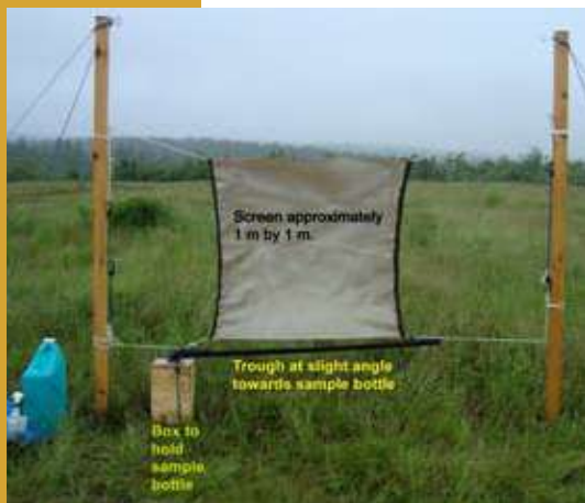
Suspended screen used to collect fog water
