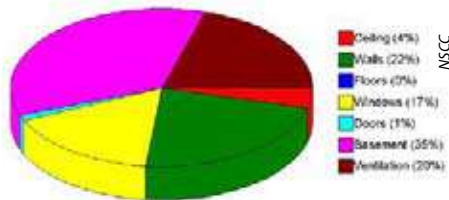
Most of MTRI's heat loss is in its basement, walls, and windows
