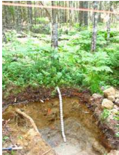
Example of granite clast till in Moose Pit catchment showing soil horizons and the water table
