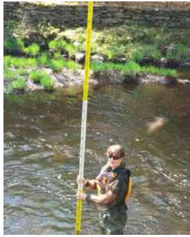
J. Eaton checks the placement of water level logger using survey equipment at Grafton Brook
