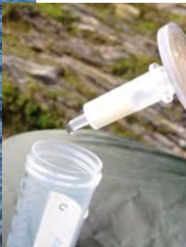
Field-speciation and separation of ionic aluminum in water samples (S. MacLeod)
