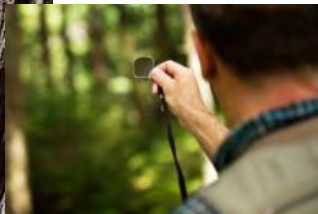
MTRI staff member, Colin Gray, using a prism to determine the basal area factor of an old forest stand (J. Headley)
