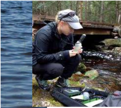
Field-crew member measuring temperature, conductivity and pH of water samples (S. MacLeod)
