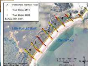
Total Station Measurements along Transects and Barrier Beach Crest (J. Woodruff)
